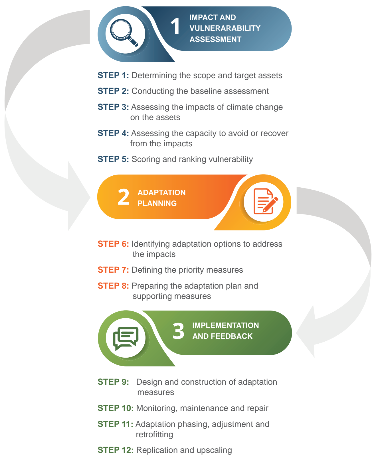
Figure 2 Phases and steps of Climate Change Vulnerability Assessment and Adaptation Planning Methodology
