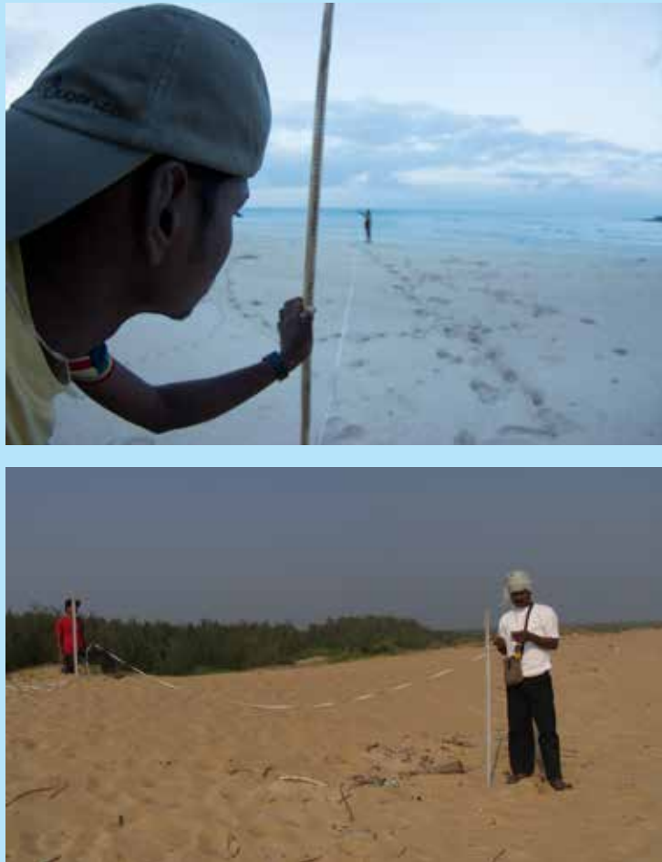
Figure 2 Emery Board Beach Mapping to Observe Beach Height with Horizon as a Level
